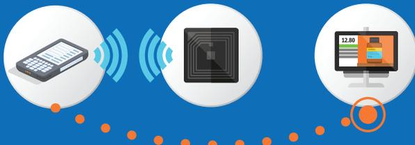
An interrogator emits a signal to the tag using an antenna. The tag responds with the information written within its memory bank. The interrogator will then transmit the read results to an RFID computer program.
